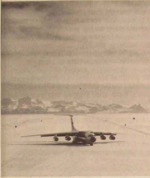
No need to haul concrete to Antarctica—Nature's 95 inches of ice withstands more than 250,000 lbs.
